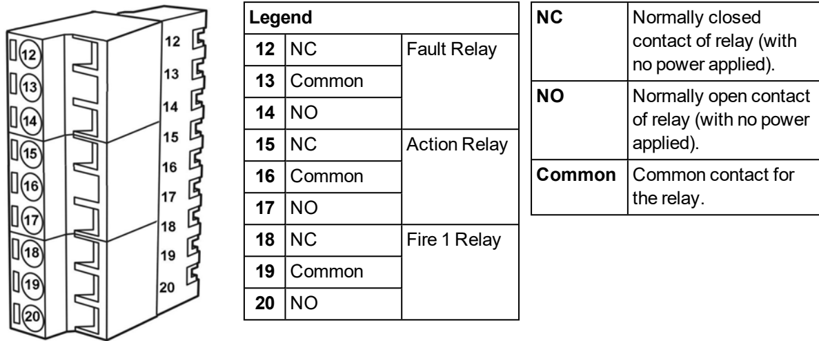
Figure 2-12: Terminal block display, relays
